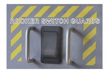
These are less common but still great to guard the rocker switches you don't want to rock by mistake, while providing oft-neglected hand stabilization. Height 3/4"; Mount on 1.5" centers with supplied 6-32 X 1/2" screws. Made of 3/16" round Aluminum alloy material.
